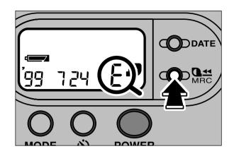
Press in the Mid-Roll Change Button. The film counter will display as it subtracts from the number of frames. When rewinding is completed, "  $\xi$  " will be displayed by the film counter.
